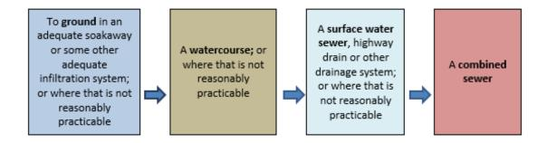
Note: in all instances adequate stormwater storage will need to be provided in order that no properties are flooded at the 100 year event (with climate change) and the there is no runoff from site from rainfall events less than 5mm depth.
